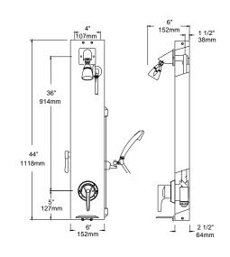
SUFFIX VX (For 104, 102 & 204 & H-15units) VX Length: To Calculate: VX Length = Ceiling height minus Shower head height minus 7 <sup>1</sup>/<sub>2</sub>" (191mm)
